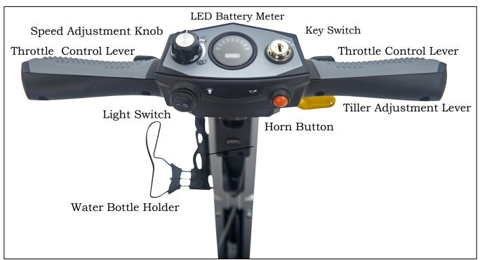
Figure 5. Carry On Tiller Control Panel
