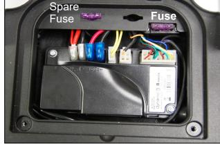
Figure 26: 35 AMP Power Module Fuse
