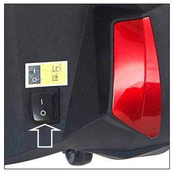
Figure 9: Freewheel Switch (Drive Position)
