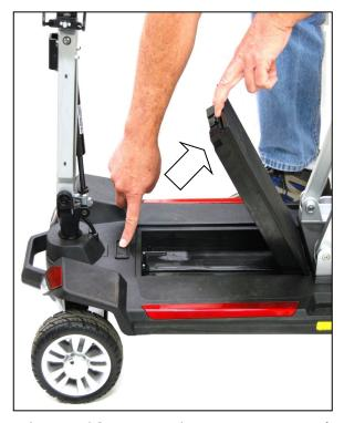
Figure 13. Removing Battery Pack
