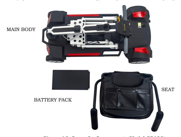
Figure 16. Carry On Components (Model GB120)
