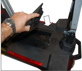
Figure 20. Installing Battery Pack
